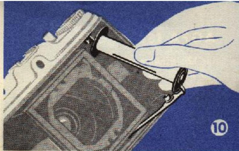
Before loading a second film into the camera the empty spool must be changed over from the left hand spool chamber to the right. The flange with the slotted hole must be engaged with the driving key of the spindle of the film wind knob, the pin of the spool holder introduced into the lower, plain hole of the spool and the spool holder swung back into the chamber.
