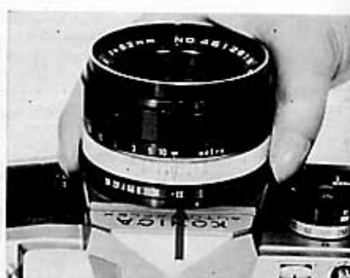
2 Set the EE mark of the aperture ring 14 to the index mark
