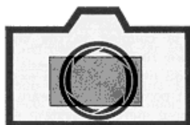
The diaphragm returns to maximum opening.
