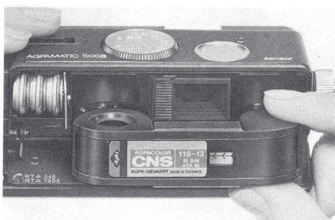
Insert the pocket cartridge as shown. The film speed is automatically set. Close the rear cover of the camera.
