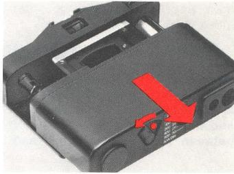
Load – or unload your Minox 35 EL in subdued light; if there is no other shade, turn your back toward the sun. Turn the back cover lock to the left so that the red dot becomes visible; slide the back cover off the camera. Insert the film cartridge into the film chamber with the protruding film end pointing to the right.
