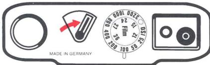
DX coding: Film speed from ISO 25 to ISO 3200 is read by the DX scanner. Non DX-coded film will default to ISO 25 setting. As a memory aid the film speed and the number of exposures should be set at the film speed reminder dial.
