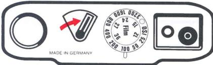
DX coding: Film speed from ISO 25 to ISO 3200 is read by the DX scanner. Non DX-coded film will default to ISO 25 setting. As a memory aid the film speed and the number of exposures should be set at the film speed reminder dial.
