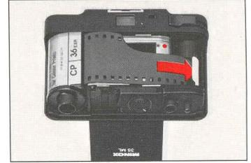
Insert the film cartridge (26) to the left of the film track with the film leader pointing to the right.
