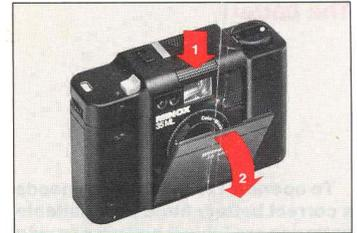
Closing the front cover retracts the lens (16), covers the finder window (10), locks the shutter release (3) and switches off all circuits.
