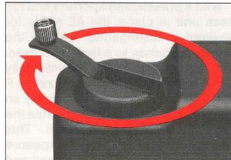
Unfold the rewind crank end with the light dot (11), in the camera top at the left.
