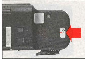
Check that the frame counter (1) is in loading position (black dot before 0). If not, press the key (9), open the front cover, operate the film transport lever till it locks and press the release button (3).
