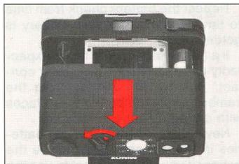
Swing over the back cover locking lever (25) in the camera base to uncover the recessed red dot, then pull off the back from below.
