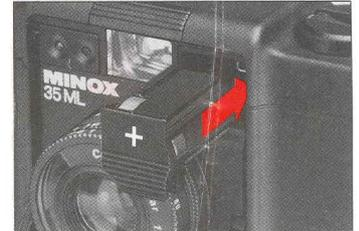
Push back the battery holder with the battery into the camera and let it engage.
