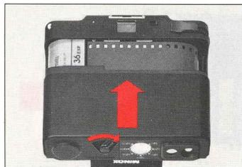
Replace the camera back by pushing it on and lock by turning the locking lever (25) to cover the red dot again.
