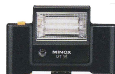
Minox MT 35 with vario-computer and tilt-up reflector: GN 26/85 (m/ft) for ISO 100, series thyristor, battery check.
