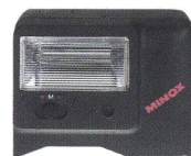
The Minox FC-E flash (with series thyristor): GN 18/58 (m/ft) for ISO 100, two aperture options for auto mode.
