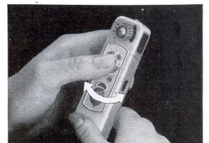
Place thumb on shutter speed dial, hold index finger under camera, turn camera with other hand
