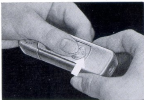
Setting the distance scale. Arrow points to sharpness zone bracket.
