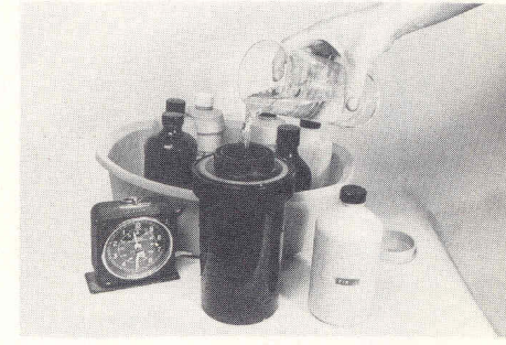
Step 15. Fix. Pour in . . . start clock . . . agitate. When time up, return to bottle.
