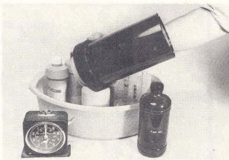
Step 5. Agitate the tank. This is done by inverting it every so often. The exact amount of agitation required will be given in the instructions for the chemistry. Be sure to hold the sealing lid on with the fingers in case it should come loose.
