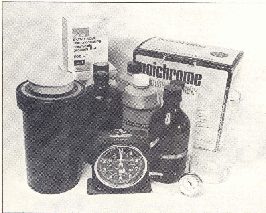
Items required for colour slide processing: Developing tank, several bottles, measure, thermometer and clock. The number of bottles you will require for the chemicals depends on which process for use. For example, the Kodak E-4 process will need nine, whereas the Unichrome process only needs seven. The extra two for the E-4 are for two additional preliminary steps, Prehardener and Neutraliser.
