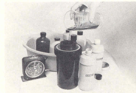
Step 13. Bleach. Pour in . . . start clock . . . agitate. When time's up, return to bottle.
