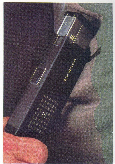
Sonocon Camera, by Minolta, 1962, unites 16mm camera, transistor radio in a nearly perfect disguise.
