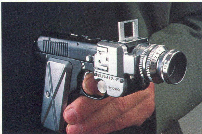
The Doryu II Flash Camera, another Japanese model for the novelty trade rather than the serious spy, has realistic clip that is loaded with flash "bullets."
