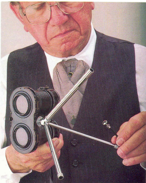
Jack Naylor attaches tripod to Stereo Photo Binocle Camera made in Germany in 1899, sold as a "detective camera."
