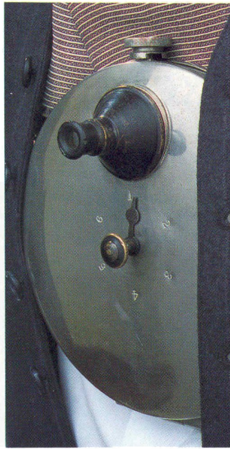
The Concealed Vest Detective Camera, 1886, worn under waistcoat, lens in buttonhole.
