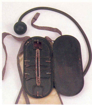
Mechanism of cravat camera (left) has a tiny chain to rotate plates for six pictures.
