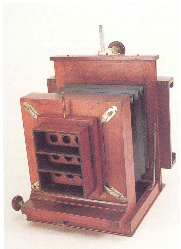
Yankee Multiplier, 1870, has nine lenses and device in back that moves a plate to take 525 tiny tintypes.
