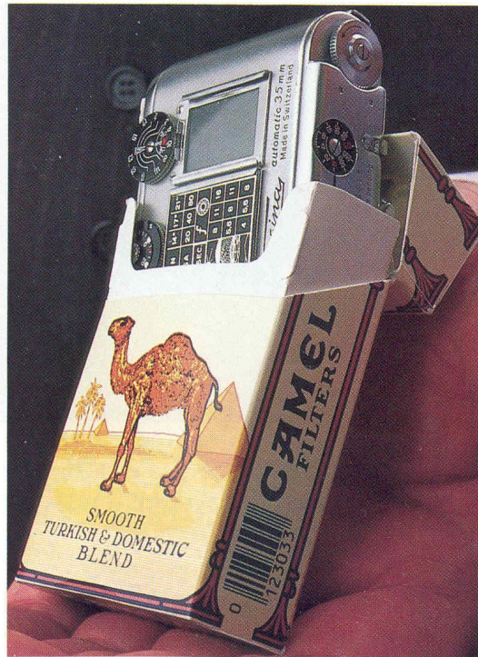
Cigarette-pack camera, a Swiss Tessina 35mm twin-lens reflex, was designed about 1960 and used by "spies" in Watergate break-in.
