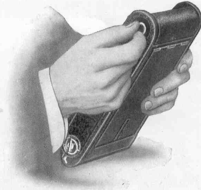
Fig. 3. Drawing out the spool pins
