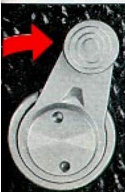
Lever pointing outwards: Field of view for 35mm lenses.
