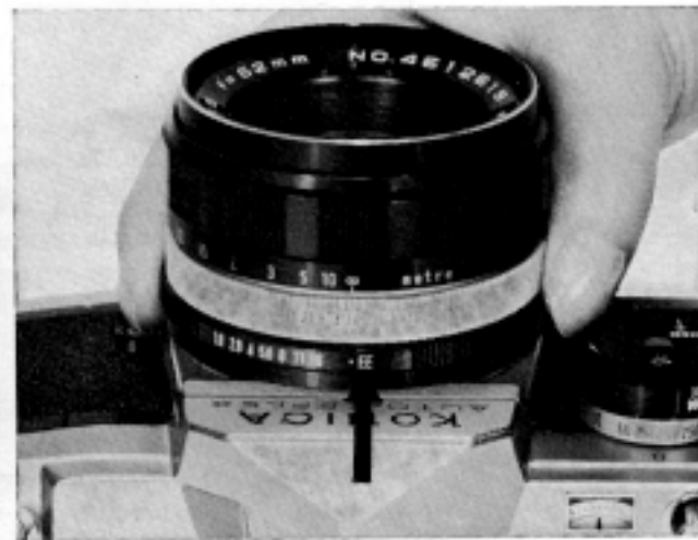
② Set the EE mark of the aperture ring ④ to the index mark
