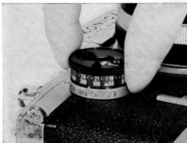
① Set the film speed scale ②③.
