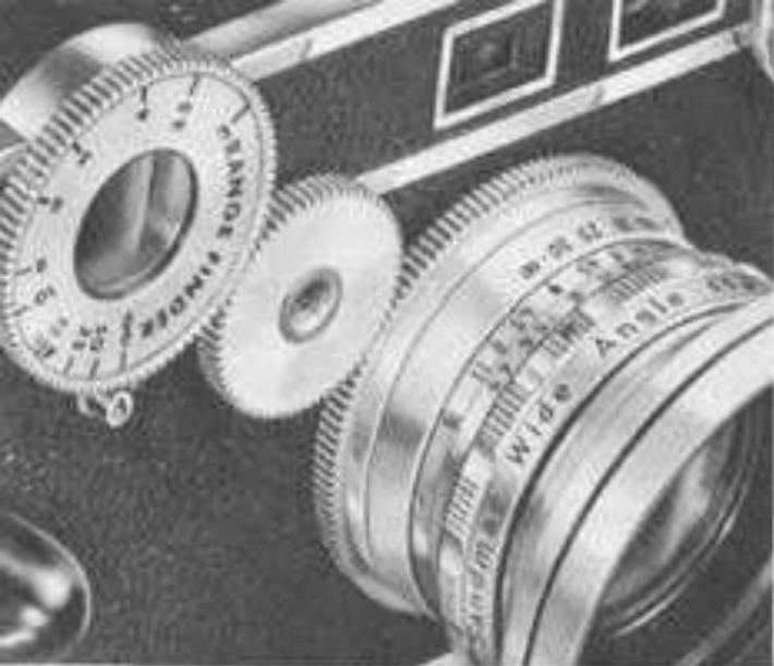
The Argus Optical Viewfinder, supplied with the Wide Angle Lens, slips into the C3 accessory shoe and provides exact fields of view for both the Wide-Angle and the Telephoto Lenses.
