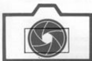
The diaphragm closes down to the f/stop designated by Electric Eye and the shutter clicks.
