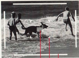
Measuring field of the rangefinder 105mm bright-line frame 35mm bright-line frame
