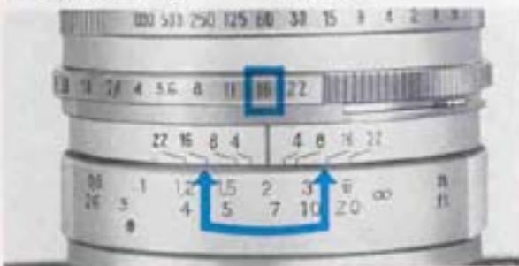
Aperture set at f/1.8 Objects in the back-ground appear blurred and out of focus. Aperture set at f/16 Objects in the back-ground appear sharply focused.
