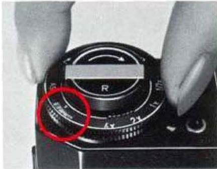
The ASA film speed is given in the data sheet packed with each roll of film. The higher the ASA number, the more sensitive the film.
