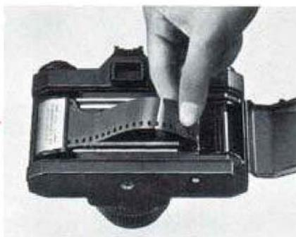
2. Place the film cassette properly into the cassette chamber, and push down the rewind knob. Insert the film leader into the slot of the take-up spool.
