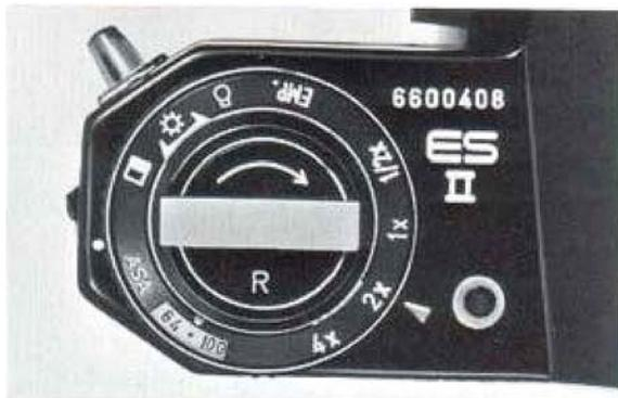
Use this control only when necessary to give intentional over- or under-exposures within the range of these factors while working on "AUTOMATIC". For example, set the dial at 2x or 4x when shooting against the light, and at 1/2x against dark backgrounds. In addition, the dial can be set between the indicated positions to achieve more specific exposure control.
