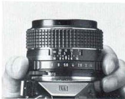
The shutter speed of the ES II is automatically determined at any speed within the range of 8 to 1/1000 sec. according to the brightness of your subjects.
