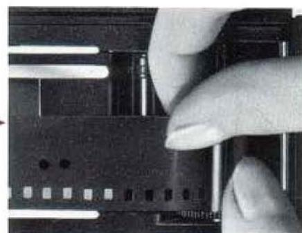
3. Advance the film by alternately turning the rapid wind lever and depressing the shutter button until both sprockets engage the film perforations properly. Close the back by pressing it firmly.
