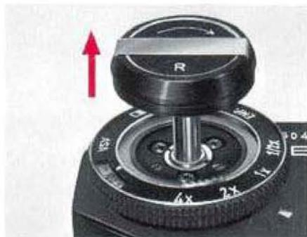
1. Open the back by pulling out the rewind knob until the back cover snaps open.
