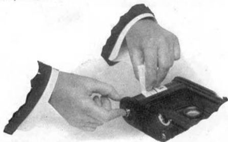
Fig. 4a. Pressing home the spool pins.
