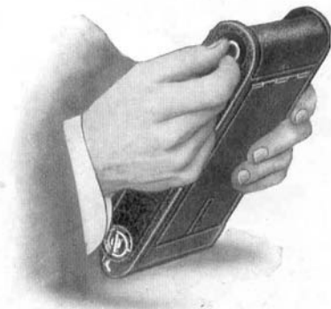
Fig. 3. Drawing out the spool pins
