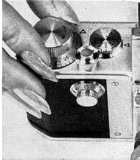
3. Turn the film winding knob.
