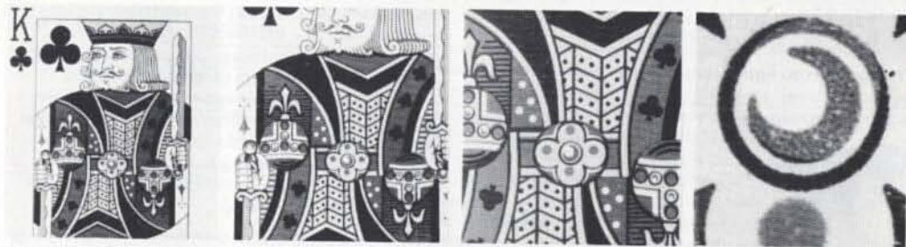
First three pictures show effect of each single tube, fourth picture shows bellows used at maximum setting.
