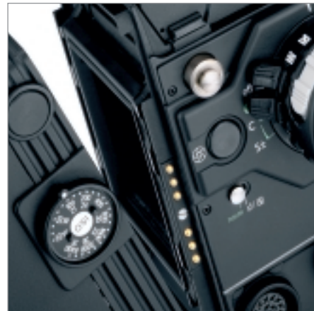
Gold contacts for reliable signal transmission/communication
