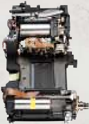
Rear chassis — film rewind and shutter charge mechanism
